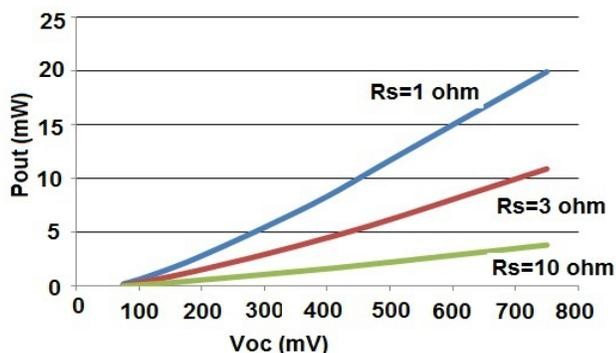
Figure 6 – Power Output vs Voc for VB0815 (Silver)
