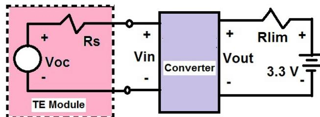
Figure 4 –Measurement Set-up for Performance Curves
