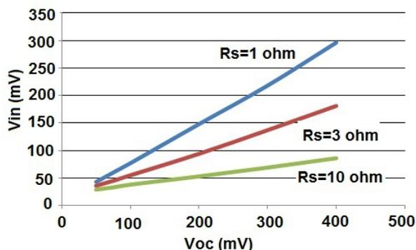
Figure 8 – Vin vs Voc for VB0410 (Gold)
