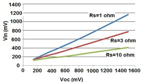
Figure 10 – Vin vs Voc for VB1299 (White)
