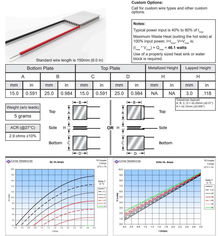
Charts above are tested at a  $T_{\mu}$ =27°C. At higher  $T_{\mu}$  temperatures, TEC resistance increases. Since V=I\*R, expect amperage to decrease for a given fixed voltage.
